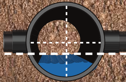
New larger HDPE pipe with raised connection point
